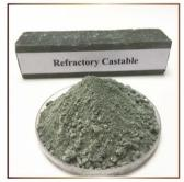
Refractories are non-metallic materials that can retain its strength and properties also when they are exposed to environments at very high temperatures that can be more than 1000° Fahrenheit. Refractories are made up of natural and synthetic materials, which is most often nonmetallic, or of combinations of compounds and minerals such as alumina, bauxite, fireclay, dolomite, chromite, magnesite, silicon carbide, zirconia and others.
